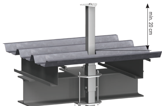
Example of pole mounting to I-beam under the roof
